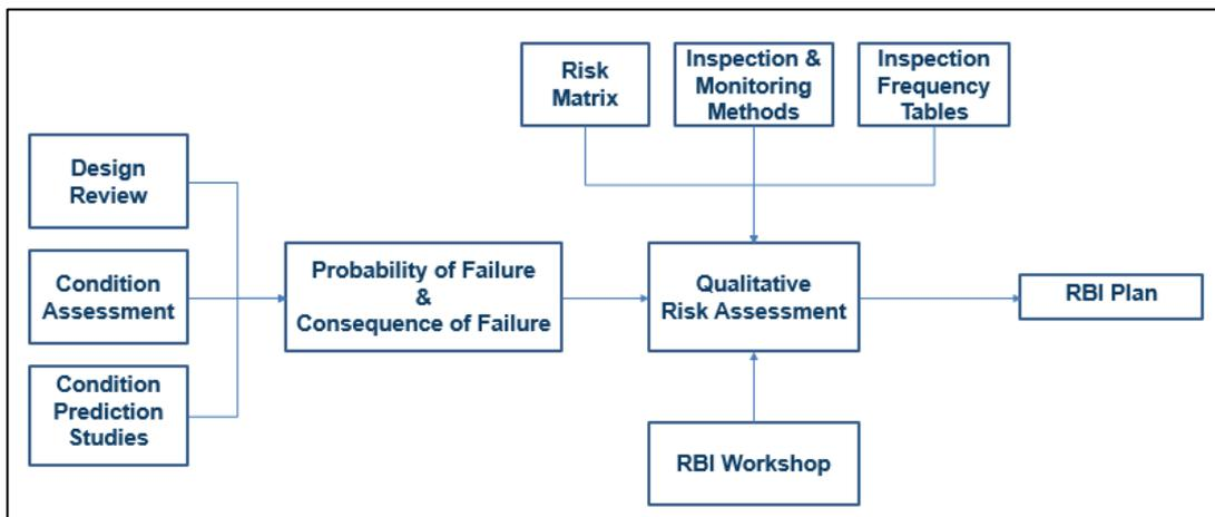
Figure 6 Simplified hull RBI development process flowchart
