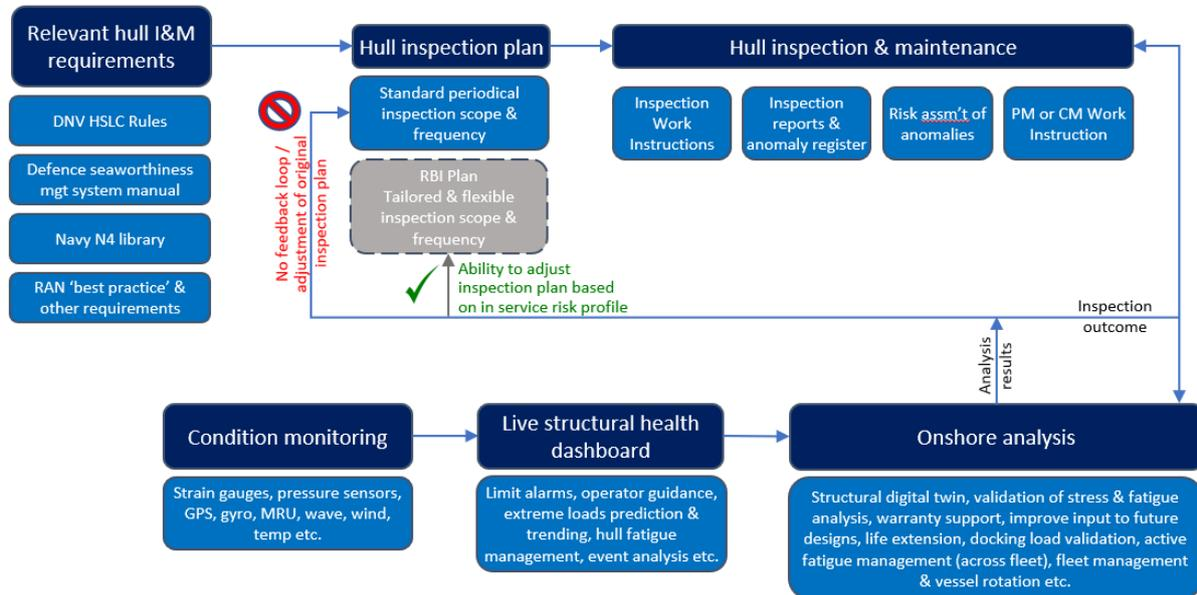
Figure 8 Example hull integrity management framework for RAN Patrol Boat
