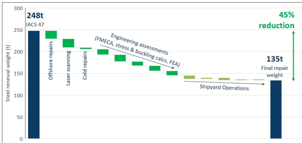
Figure 7 Inspection and engineering optimisation – repair steelweight waterfall chart
