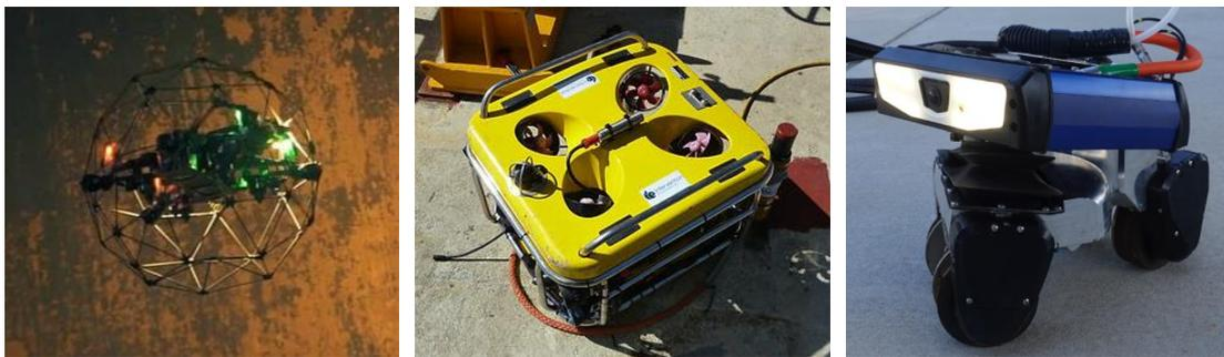
Figure 2 Example of a UAV [9], an ROV [10] and a crawler [11] used for hull structure inspection
